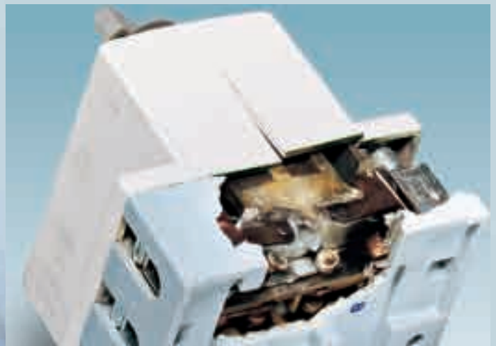
Fig. 1b: Destroyed residual current circuit breaker (RCD)
