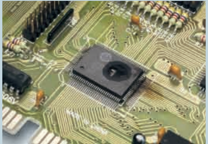
Fig. 1a: IC destroyed by surge voltages
